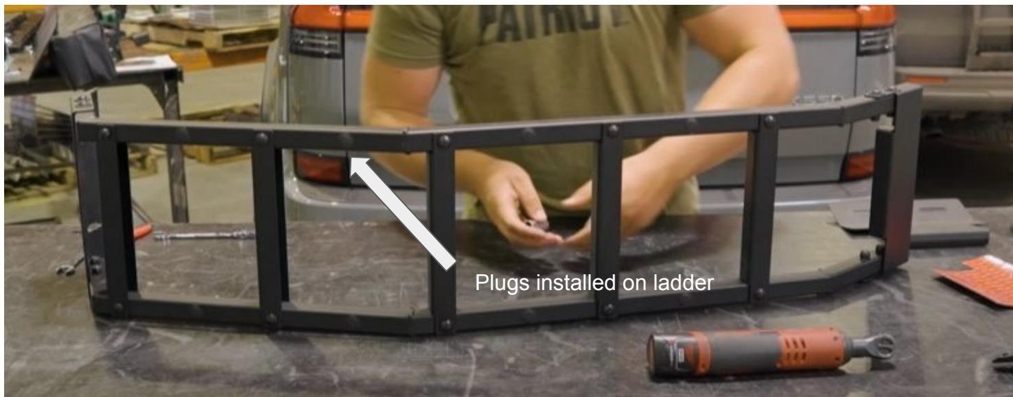
Place the ladder side rail plugs in the rung locations that are not being occupied.
