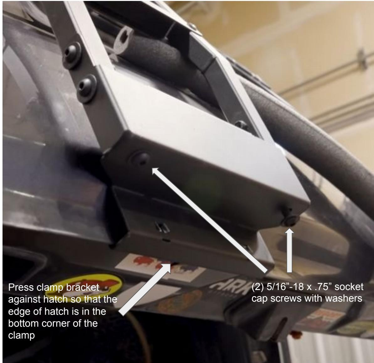
Place the last strip of 3m adhesive pad onto either side of the clamping plate. Then remove the other side of the adhesive backing in preparation for the final step.
