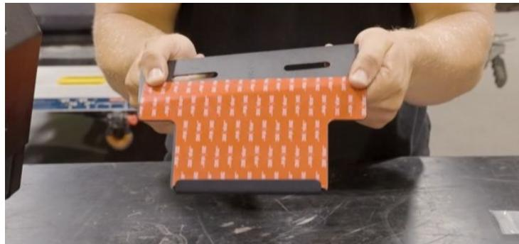
Place the ladder on the vehicle and hook the top bracket onto the hatch. From here you're going to **MEASURE (9 5/8")** from the corner of the hatch adjacent to the roof track on the roof of the vehicle, to this specified edge on the top hatch mounting bracket. From there, mark this location with a piece of painters tape to remember the location.
