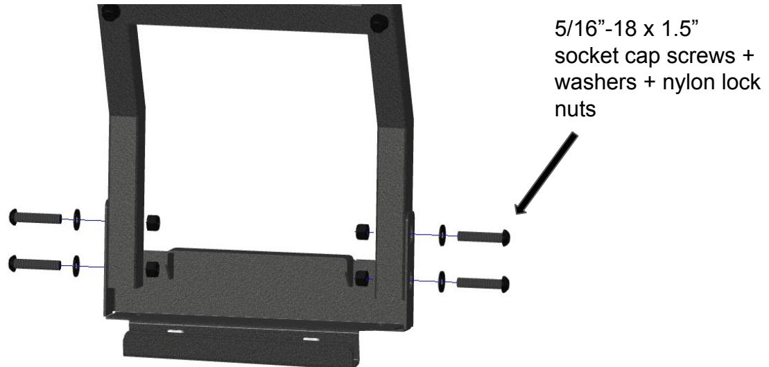
Apply (2) smaller 3m adhesive strips to the clamping area that will come in contact with the outside of the vehicle rear hatch. Then, press the cage nuts into the square holes on the inside of the clamping area of the bracket.
