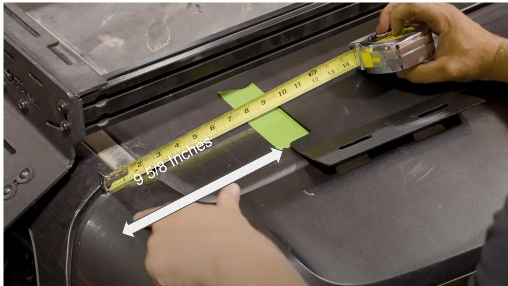
Remove adhesive pad backing on the top hook bracket, and locate the top hatch mounting bracket in the marked location with the tape.
