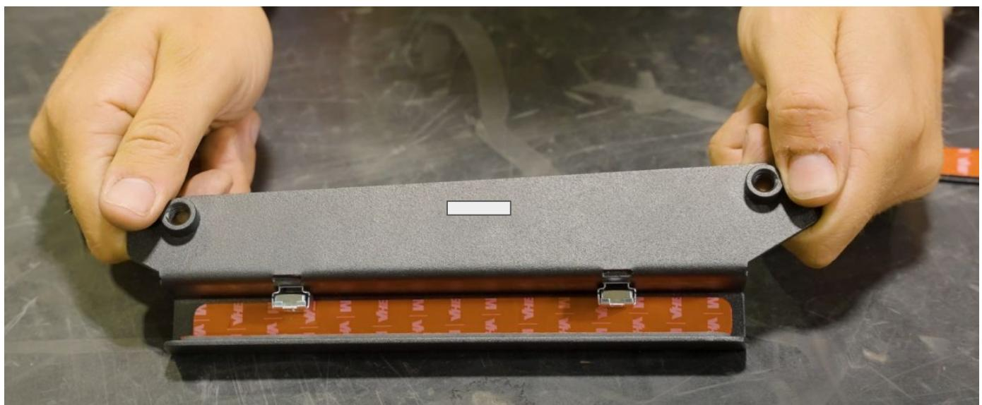
Once the ladder is level vertically, remove the other side of the adhesive backing of the 3m pads on the clamping bracket and press the adhesive pad onto the inside of the hatch.
